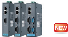
EKI-1220 Series 1/2/4-Port Modbus Gateway/Router
